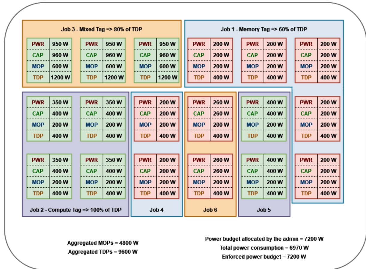
Figure 37: Example of power budget sharing for a partition of nodes completely loaded by the execution of six jobs, according to the Application-Aware Power Capping (AAPC) mechanism..
